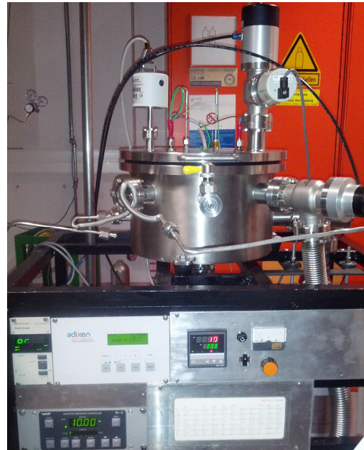
Fig. 1. (left) Design of the PECVD reactor and, (right) picture of the system.
