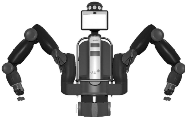
Fig. 3 – Baxter robot by Rethink Robotics, with 2 mirrored 7 degree of freedom arms.
