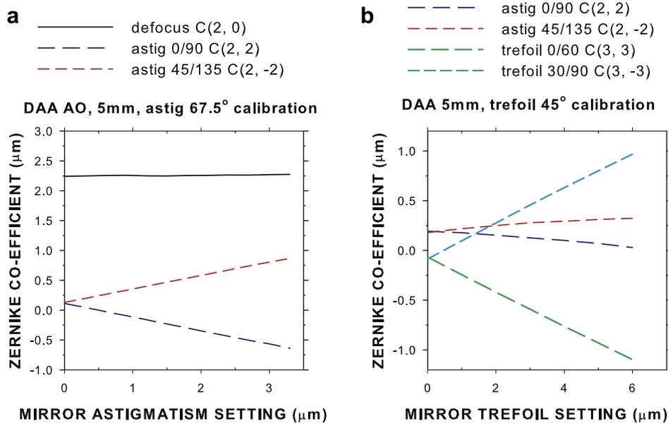
**Fig. 2.** Main changes in aberration coefficients with change in mirror setting for subject DAA for (a) astigmatism with instrument meridian  $67.5^\circ$ , and (b) trefoil with instrument meridian  $45^\circ$ . Note that coefficients are not zero at the zero mirror setting; this is because of adjustments of the system to correct the subject's aberrations, either with the optical trombone (defocus) or with the mirror (astigmatism, trefoil).
