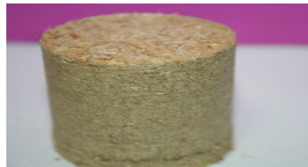
Fig 5. Detail of a briquette from Miscanthus powder
