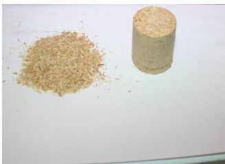
Fig. 4. Initial material and briquette obtained
