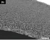
Figure 1: Scanning electron micrographs of the (a) inner surface and (b) cross-sectional cryogenic fracture of the plasma filtration hollow fiber membrane in Plasmylane 6. Scale bar represents 10  $\square$ m.
