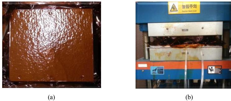
Fig. 2. The process of sample prepared by hot press: (a) vacuum packaged and (b) curing in hot press
