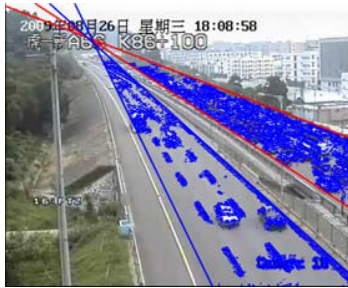
Fig. 3. Edge pixels in road areas of Figure 2(a).
