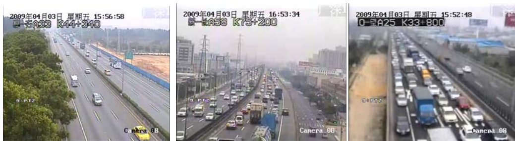
Fig. 6. Three typical traffic state scenes. (a) Smooth state; (b) Slow state (right lanes); (c) Congestion state (left lanes)
