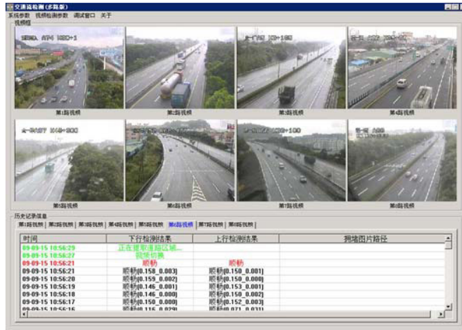
Fig. 8. Software interface of traffic state detection system
