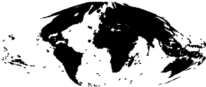
Fig. 3. Global land grid defined by 9233 unique non-Antarctic land Landsat WRS path/rows defined the U.S. Landsat project "Land Definition" data base and from the geographic corner coordinates for these path/rows extracted from the 2000 and 2010 epoch Landsat TM and ETM+ metadata. The grid is defined in the sinusoidal equal area projection and is composed of 6,138,864 land grid points spaced every 5.559752 km in the X and Y axes of the sinusoidal coordinate system.
