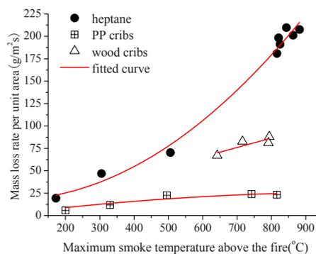
Fig. 4. The influence of smoke layer temperature vs. different fuel combustion rates.
