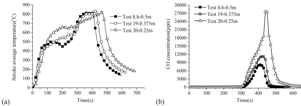
Fig. 5. Influence of opening size on fire development. (a) average gas temperature in comparison (section A); (b) CO concentration in comparison (section E).
