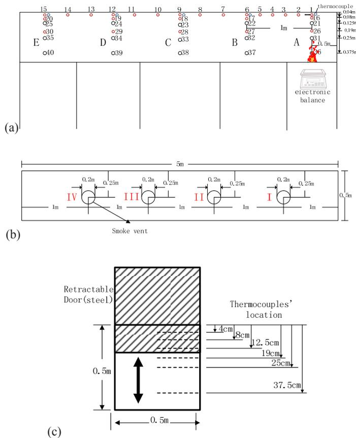
Fig. 1. Geometry of the experimental set-up. (a) longitudinal section view; (b) top view; (c) cross-section view.
