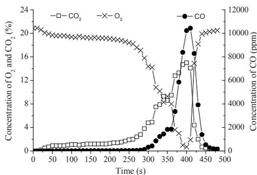
Fig. 3. Variation of smoke density vs. time (test 8, section B).
