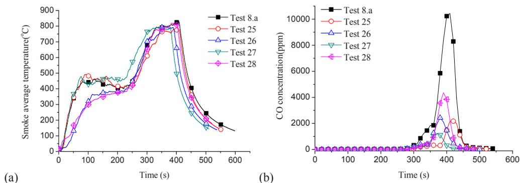
Fig. 6. Influence of transverse ventilation on fire development (a) average gas temperature in comparison (section A); (b) CO concentration in comparison (section B).
