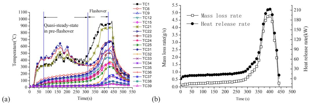
Fig. 2. Results of test 7. (a) variation of temperature vs. time; (b) variation of mass loss rate and heat release rate vs. time.
