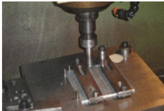
Figure 1 FSW setup showing work piece and Backing Plate
