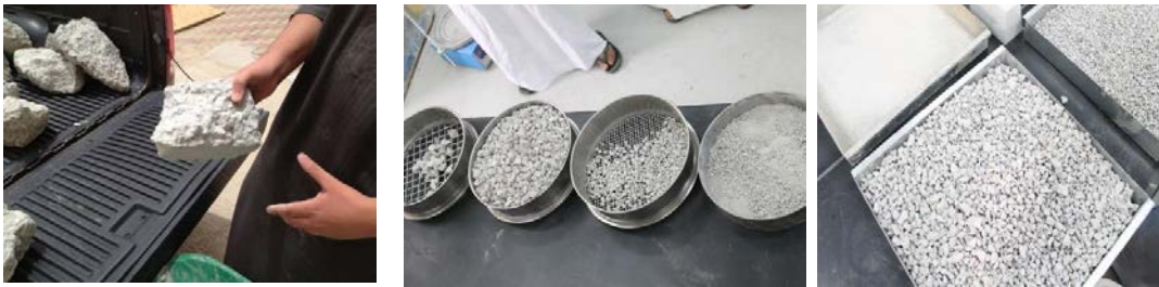
Fig 2: Processing construction debris into gravel.
