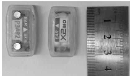
Figure 1. Wireless sensor used to measure head impacts during un-helmeted play.
