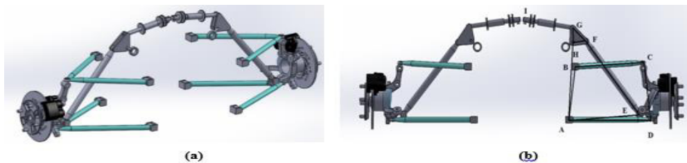
Figure 2. Front Suspension (a) Isometric view (b) Front view with labelling
