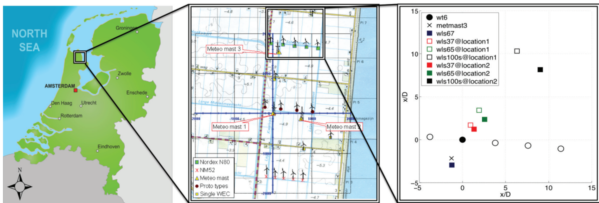
Fig. 1. a) Map of the Netherlands with a black box indicating the location of ECN's wind turbine test site Wieringermeer. b) Map of the wind turbine test site with a box indicating the row of research turbines. c) Map of the WINTWEX-W measurement setup around the research turbine number 6.
