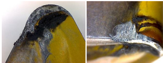
Fig. 3. Wear on rake face and flank face of carbide cutting tools after roughing.
