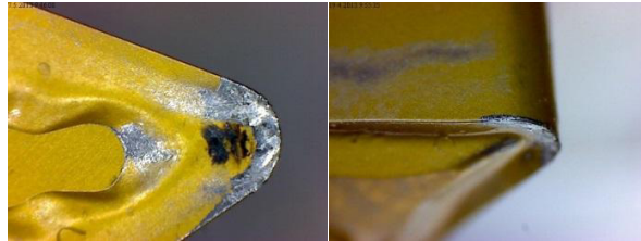
Fig. 5. Wear on rake face and flank face of carbide cutting tools after finishing.
