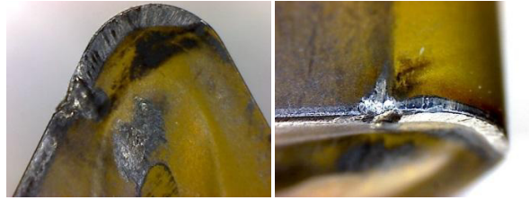
Fig. 4. Wear on rake face and flank face of carbide cutting tools after semi finishing.
