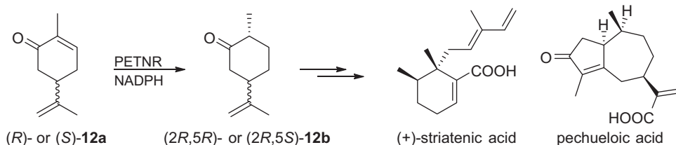
Fig. 4. Total asymmetric synthesis of striatenic and pechueloic acid via ene-reductase catalyzed reduction of carvone 12a producing the key intermediate 12b .
