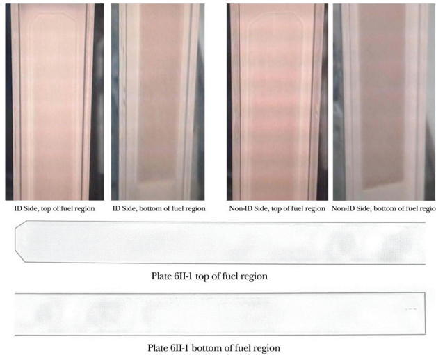
Fig. 15. Postirradiation Visual Examination (Top) and Ultrasonic Examination (Bottom) of AFIP-6MkII Fuel After Irradiation to 4.3 \times 10^{27} f/m 3 at a Peak Power of 35 MW/m 3 . No Indications of Delamination, Blistering, Warping, or High Swelling were Observed.
