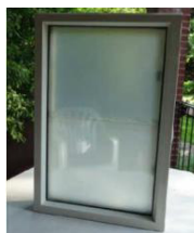
Fig.2. 3-glass aerogel transparent window (890 x 580 x 110 mm): Frame-Thermopane
