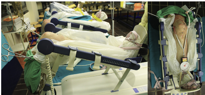
Fig. 3. The lower limb is strapped to a CPM device to perform 60 motion cycles of 90 s ( 0^\circ – 90^\circ – 0^\circ ) (left). To simulate partial loading elastic straps are stretched between a Steinman pin in the distal femur and the foot, and a force transducer is incorporated to control the 15 kg force applied between the two joints (right).
