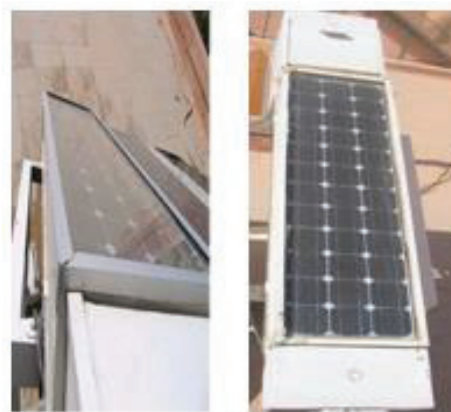
Fig. 6 Photograph of the prototype of hybrid PV/T air collector at URAER Unity, Ghardaïa.
