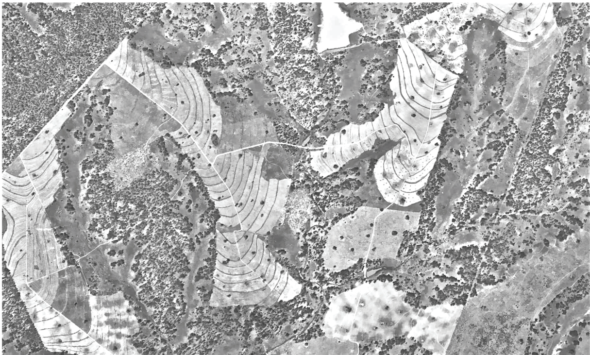
Fig. 6 Vertical overhead view of part of a developed tobacco farm ( elsewhere, but on similar landscape to that in Figs. 4/5 ), showing crest-roads and contoured layout of fields on land-type suitable for tobacco production. The remaining areas, judged as unsuitable, being too wet/ too sandy/ too steep, were allocated as grazing-land for cattle. Black spots are termite-mounds.
