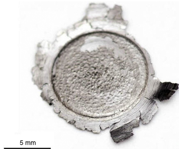
Fig. 2 – Sample processed by quasi-constrained high-pressure torsion.
