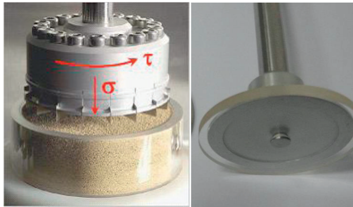
Fig. 1. Image of the shear cell supplied with the FT4 powder Rheometer (a) measuring powder flow functions; (b) measuring angle of wall friction
