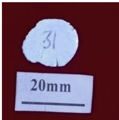
Fig. 3. Schematic of the deformed specimen tested at a strain rate of 4500/s.
