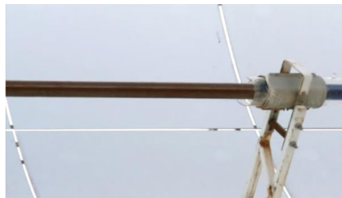
Fig.1. Typical picture of a broken glass cover due to bending of absorber tube
