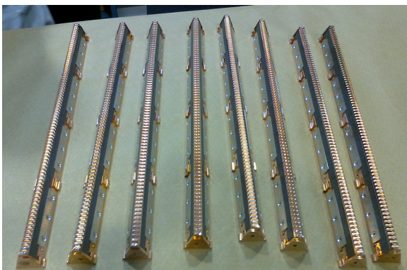
Fig. 3. PETS assembly, copper rods with the SiC ceramics positioned along the prism sides.
