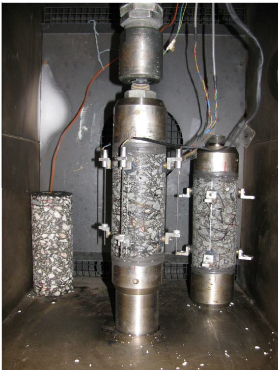
Fig. 2. Instrumented specimen ready for testing within environmental chamber.
