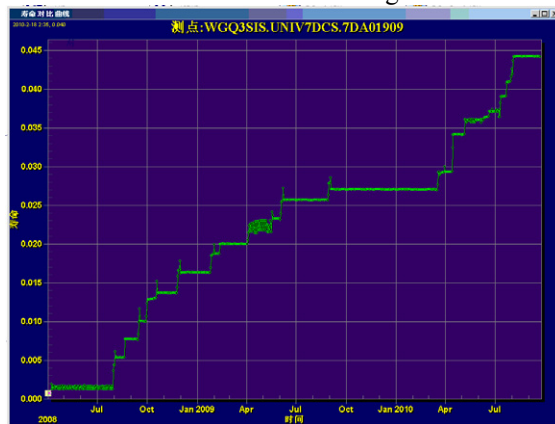
Figure 7. Life curve drawn by Assessing System for Life of HP heaters
