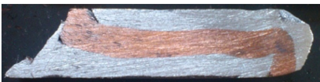
Fig. 2. Tri-layer specimen after four ECAE passes.
