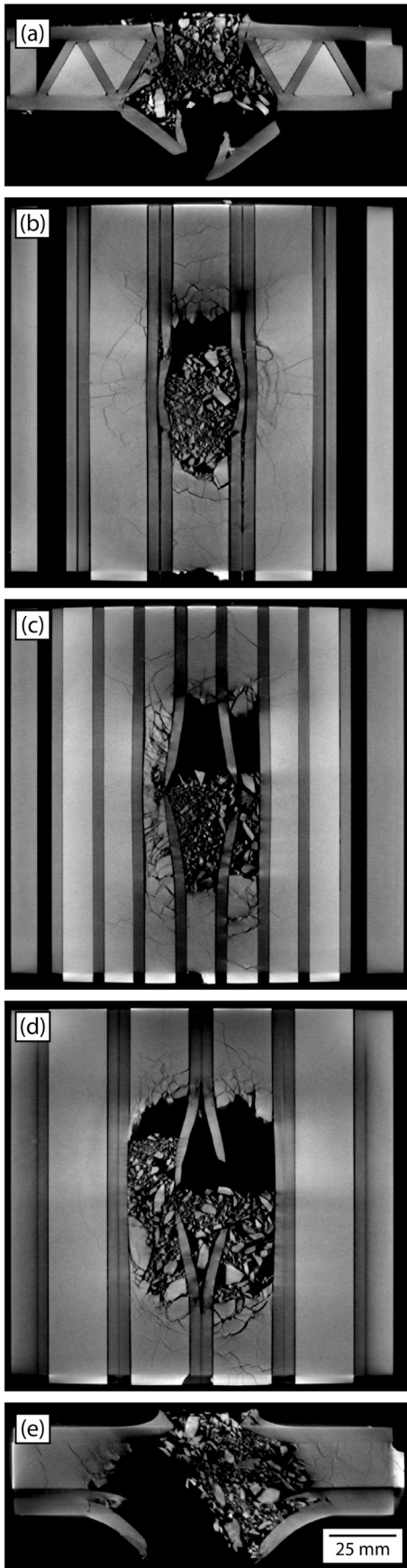
Fig. 11. XCT cross-sectional views of a base impacted panel. The projectile's impact velocity was 1492 \text{ m s}^{-1} .
