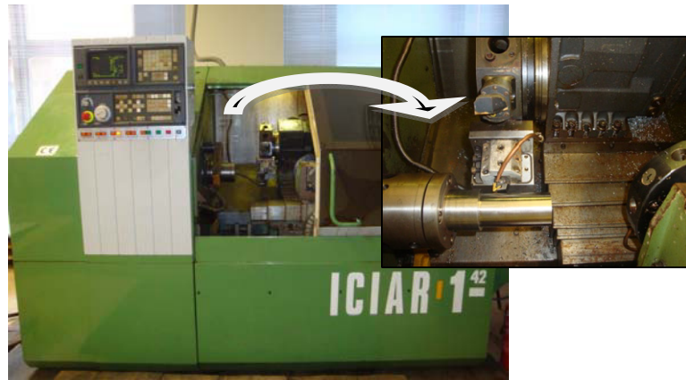
Fig. 3. Mupem lathe with dynamometric plate.
