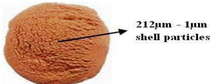
Fig. 1 Photomicrograph of raw wood apple shell particles
