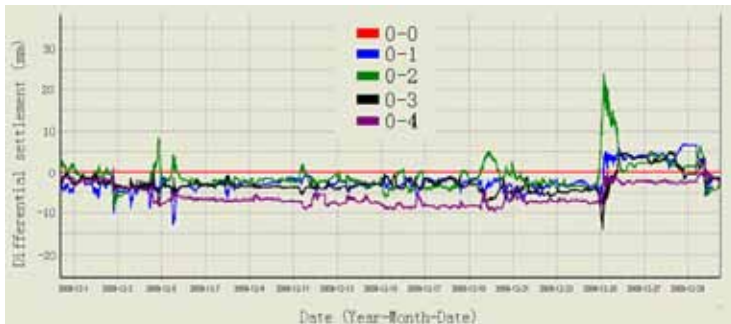
Fig. 6 Differential settlement curves during the whole monitoring term
