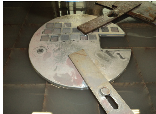
Fig. 2 Experimental set-up; the inconel plate is clamped onto the AWJ table and pockets are cut
