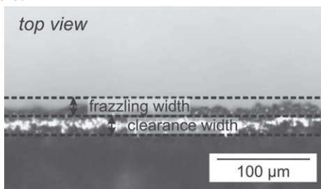
Figure 6. Scheme of the determination of characteristic values for the cutting quality with the aid of a top view of the cutting edge
