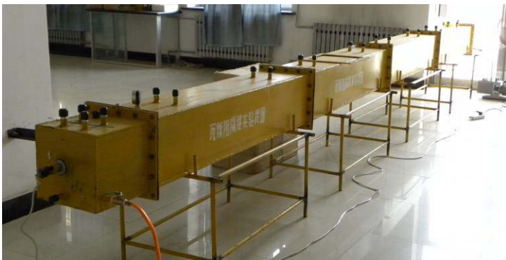
Fig. 2. the figure of the experimental pipeline
