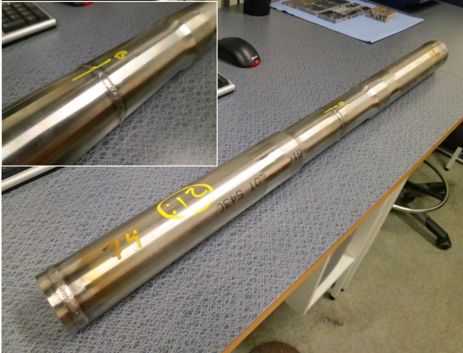
Fig. 1. Finished test specimen after joining the separate machined pipes with a welding joint. The insert represents a close-up view of the circumferential butt weld, in as-welded condition.
