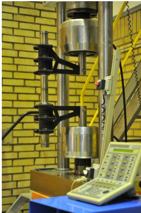
Fig. 2. Experimental set-up for fatigue testing of the piping components.
