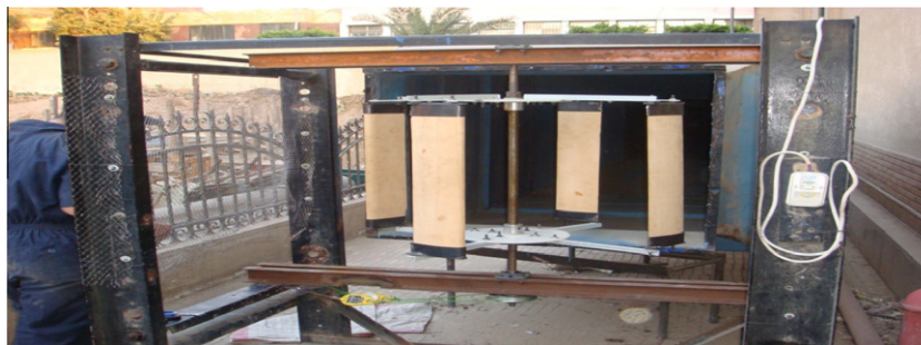
Figure 3a Turbine and test rig photo.
