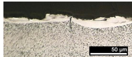
Fig. 4. Example of crack occurrence in the remelted layer (Poco EDM-3 cathode, 220 V, 15 A, 0.12 duty cycle).
