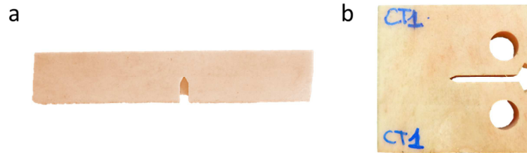
Fig.1. (a) SE(B) specimen; (b) C(T) specimen.
