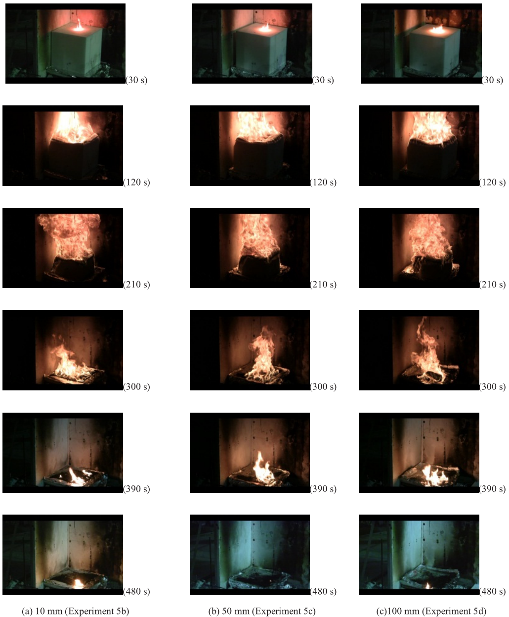
Fig. 3. Burning behavior in near-corner configurations with 10, 50 and 100 mm of separation distances.
