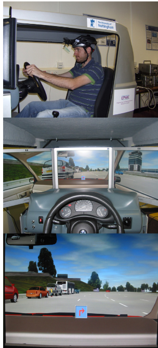
Fig. 1. The simulator used in the current study. The top panel shows a participant sat in the cab wearing a head-mounted eye tracker. The middle panel shows the three-screen display with steering wheel and dashboard. The bottom panel shows the centre screen containing a behavioural prediction precursor: a small child waits between parked cars on the left to cross the road.
