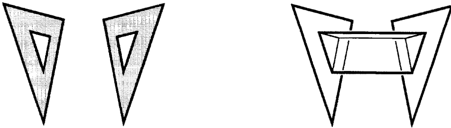
Fig. 2. The centers of two non-planar triangles are removed (left) and the holes are attached by a triangular tube (right). The resulting handle is tight and immersed.
