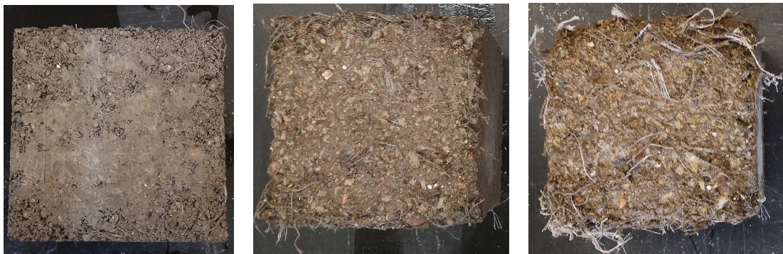
Fig. 5. Surface of specimen (a) before testing; (b) after 25 cycles; (c) after 50 cycles of freezing and thawing.
