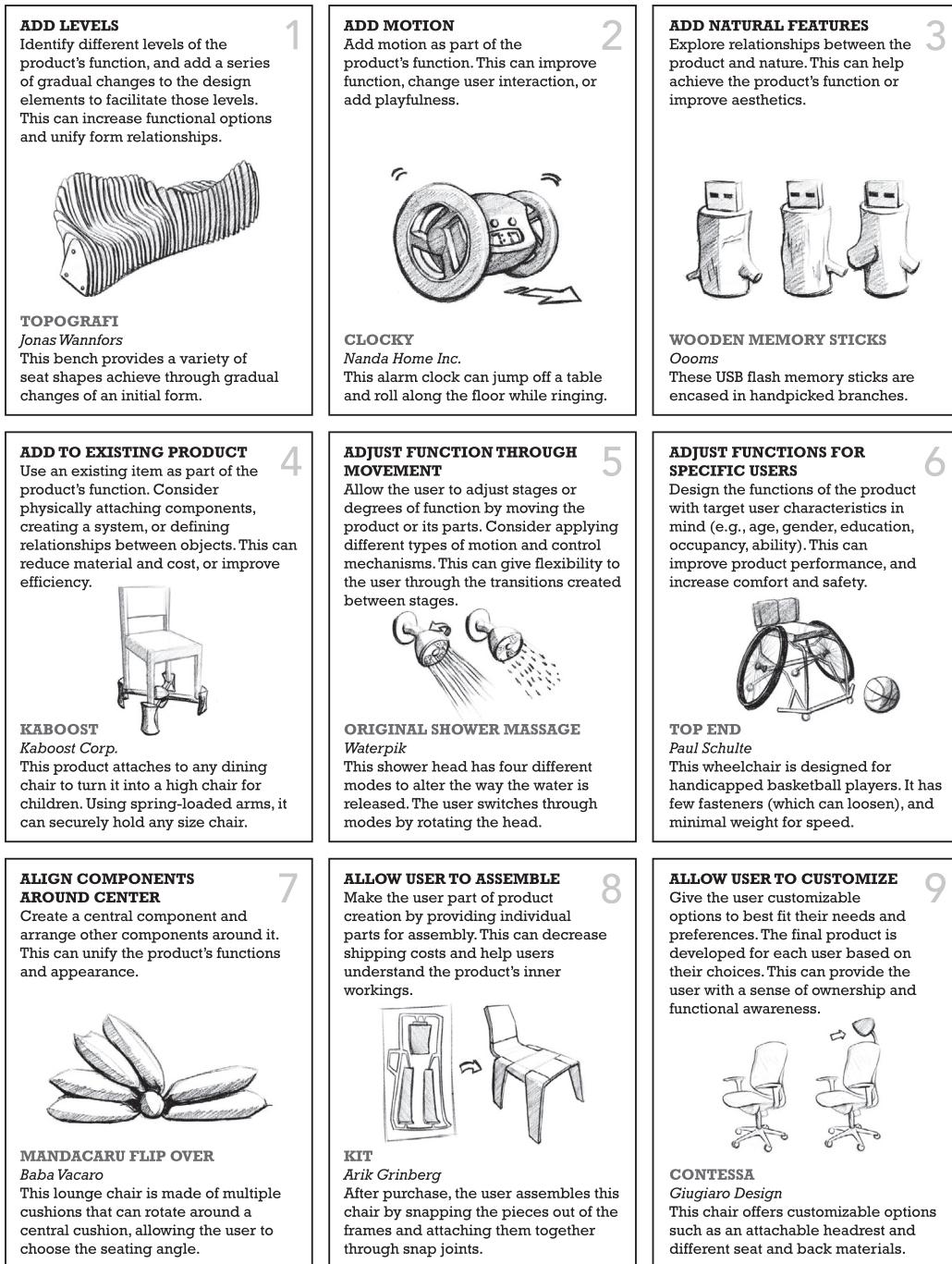
Figure 6 The 77 Design Heuristics identified across four studies of award-winning product designs, a solo professional design project, and protocol studies of engineers and industrial designers working on a novel problem. Each is illustrated with a description and an example consumer product where the Design Heuristic is evident. (Courtesy of Design Heuristics, Inc.)
