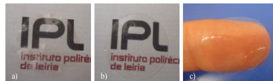
Fig. 4. Transparency of the film AGA25 in dry (a) and wet state (b), and its appearance on the human finger of a volunteer (c)
