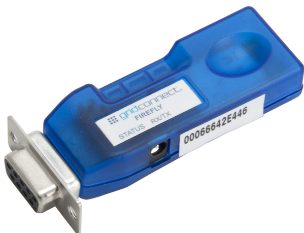
Fig 1. A Bluetooth RS232 serial adapter. Numerous such devices are available. The adapter enables the anesthesia monitor to appear as a pairable Bluetooth device on the user's mobile device. The adapters are typically Class 1 devices and have a range of about 100 meters. However, most mobile devices are Class 2 devices and have a range of only 10 to 15 meters.
