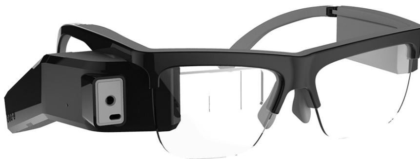
Fig 4. The Optinvent ORA-S head-mounted display. The device can be used to display information in the periphery of the wearer's visual field and is paired with the user's mobile device using a wireless connection. The device also can incorporate an audio system. The loudspeaker can be used for the sonification of physiologic data signals and the microphone for interacting with an expert system.
