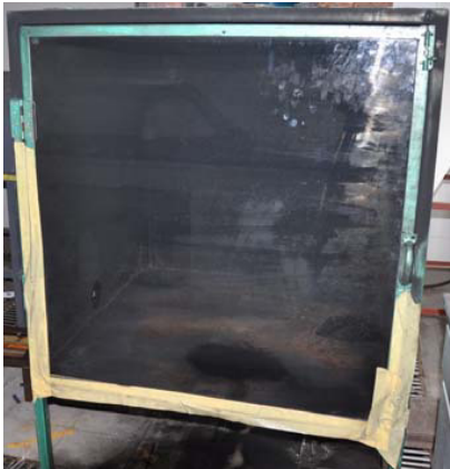
Fig. 1 The picture of the confined compartment (1m \times 1m \times 1m)
