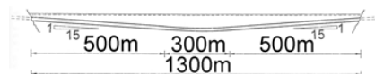
Fig. 2. Downward arched SFT between Vallavik and Bu in Eidfjord in Hardanger in western Norway [2]
