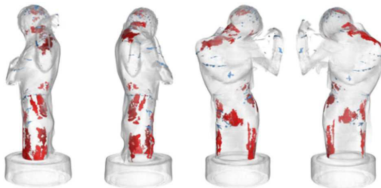
Fig. 7. Mapping showing corroded areas (in red) inside the lead sheet, remains of flux and nails (blue) according to the information given by the tomograms.
